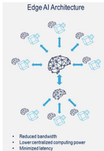
Figure 3.8. - Edge AI architecture (Source: STMicroelectronics)
