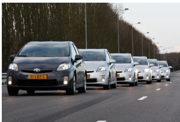
Figure 2-7: Platooning vehicles on public road, lead vehicle has driver
