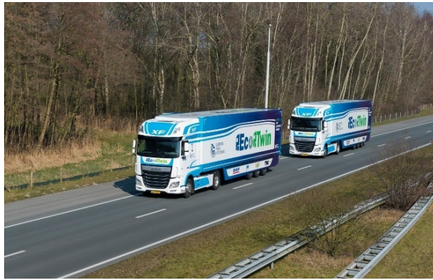
Figure 2-8: Platooning trucks on public road, lead vehicle has driver
